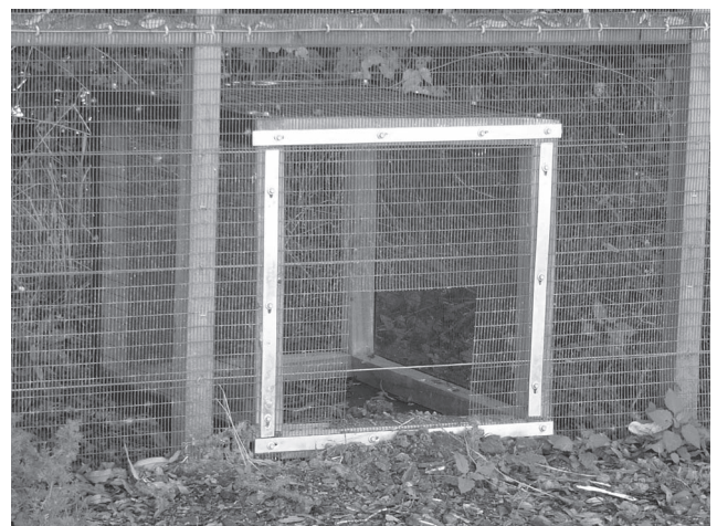
Fig. 2. An observation cage as installed at the fence. The temporary mesh cover has been removed and the simulated 'flood-scour' breach is open.
